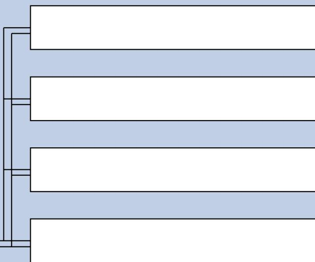
You can control up to four radiators, for a maximum power of 2000 watt, with just one receiver
